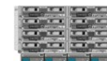
Compute 1 Cisco UCS 5108 Blade Chassis 2 Cisco UCS 2208 IO Modules Up to 8 Cisco UCS B200 M4 Blade Servers
