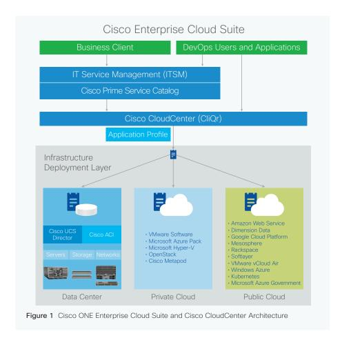
step process. These cloud-agnostic application profiles are portable and easily manageable to deliver flexibility. The Cisco CloudCenter platform grows with your organization, letting you start with one cloud environment and expand to as many environments as your business needs, with full application lifecycle management and full infrastructure lifecycle management.
