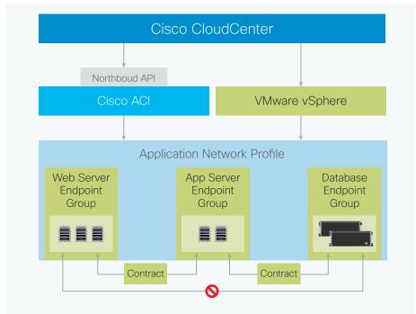
**Figure 4** Cisco ACI Creates the Network Container, Endpoint Groups, and Contracts Between the Tiers and Manages Traffic Flow for Greater Security
