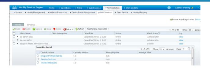
The FMC has successfully registered to the ISE pxGrid node and subscribed to the EndPointProfileMetada, SessionDirectory and TrustsecMetaData capabilities.
