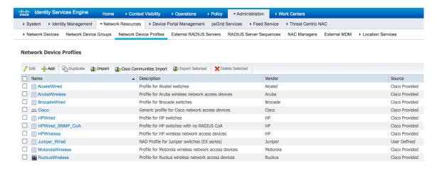
Now that the Network Device Profile is imported we can add the switch to the Network Device database and specify it as a Juniper\_Wired device. Navigate to Administration > Network Resources > Network Devices and add a new device as shown. Note the "Device Profile" selected at the bottom of the capture.
