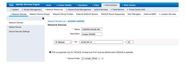
The device is now added to the database correctly as a Juniper device and we can now setup the policy for AAA functions for this device.
