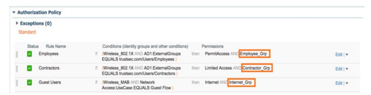
Step 3 Assign a security group to each of the Authorization rule based on the user role/device type like **Employee\_Grp** etc.
