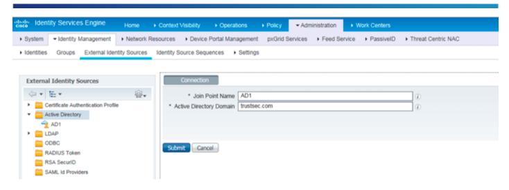
Step 1 Select all the ISE nodes and click **Join** to connect the nodes to the AD server. Provide the **AD User Name** and **Password**
