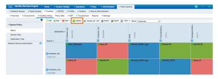
Step 6 After the Matrix is deployed look for the notifications messages (CoA) on the upper right corner. **Push** to send any configuration changes to the network devices or click **OK** to acknowledge the notification messages
