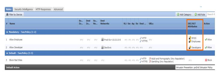
Additionally FTD provides **Rapid Threat Containment** (**RTC**) capability by detecting the threat and sharing that information over Cisco PxGrid to ISE and ISE could quarantine that endpoint using the TrustSec Security Group Tags.
