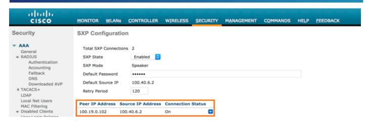
Step 10 Now enable the SXP peering between ISE and ASA with ISE as SXP Speaker and ASA as a SXP Listener to share all the IP-SGT mappings that ISE received from WLC to ASA.
