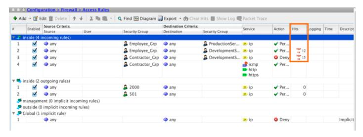
As soon as an **Employee** tries to access the **Development Server**, as per the **Permit** action configured on the access rule of the SGFW policy he would be granted network access and the number of **Hits** would be incremented. Similarly when a **Contractor** tries to access the **Development Server**, as per the **Deny** action configured on the access rule he would be denied network access and the number of **Hits** would be incremented.
