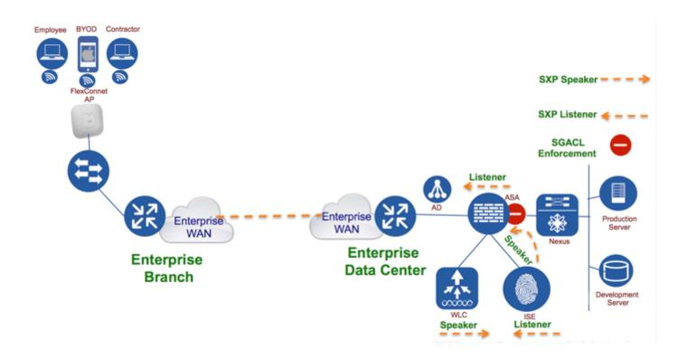
The above topology shows the SXP peering between ISE and WLC. Since ISE is acting as both SXP speaker and Listener it can not only receive the IP-SGT binding information from the WLC (SXP Speaker) but also can share the IP-SGT bindings to other devices in the network. The above topology shows ISE as a SXP Speaker sharing the IP-SGT binding information to an ASA. Here is the configuration to enable the peering between ISE and WLC.
