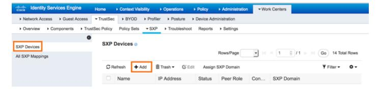
Provide the Name, IP Address, Peer Role Speaker as WLC is a SXP Speaker, Connected PSNs on which the SXP Service is running, SXP Domain which could be default domain or a custom created one, Status as Enabled, Password Type can be DEFAULT Global Password or a CUSTOM created and the SXP Version it needs to be running which is V2 for the WLC.
