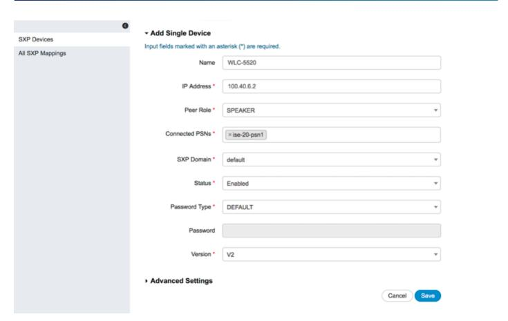
SXP Domain provides a means to logically group network devices to which SXP mappings should be exchanged. These "Domains" are arbitrarily defined and purely optional; if none are defined the system default VPN named "default" is used. This allows for granular control of where specific SXP mappings will be advertised
