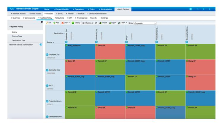
Step 5 Once the TrustSec Policy Matrix is configured click **Deploy** to push the **SGACLs** and their permissions to the network devices.
