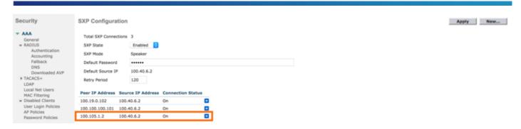
Step 19 To validate the SXP Connection status of WLC on the ASA navigate to Monitoring > Properties > Identity by TrustSec > SXP Connections
