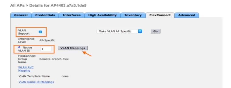
Step 5 Click VLAN Mappings to map the specific WLAN VLAN mappings used by the FlexConnect AP. Select the specific WLAN ID used by the AP and click Apply
