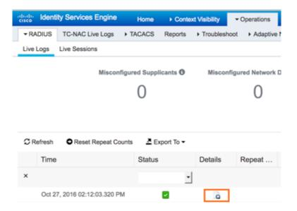
Step 9 The Live Logs Details shows the all the endpoint details including the Security Group it got assigned
