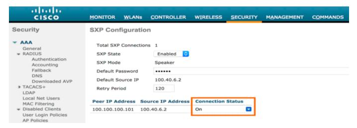
Step 5 Validate the connection status on the Cat6K with the below command. The connection version is 2 since WLC supports SXPv2
