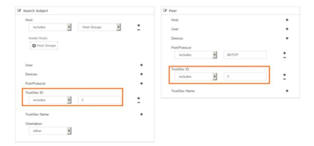
Additionally even StealthWatch can provide **Rapid Threat Containment** (**RTC**) and Network as a Sensor and Enforcer (NaaS/E) capability by detecting the threats through policy violation and sharing that information over Cisco PxGrid to ISE and ISE could quarantine that endpoint using the TrustSec Security Group Tags.
