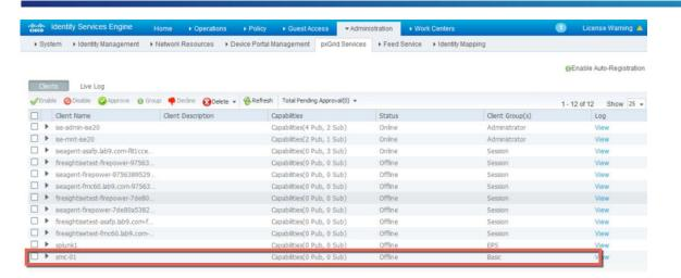
Step 9 Move the registered Lancope smc-01 client to the EPS client group. Select smc-01->Group->delete Basic, select EPS->Save
