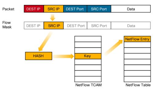
Figure 4. NetFlow Hash Operation
