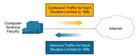
Figure 7. Bidirectional UBRL Scenario Example
